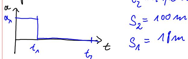
$$v_{max} = a \cdot t_1 = \left( \frac{2s_1}{t_1^2} \right) \cdot t_1 \Rightarrow t_1 = \frac{2s_1}{v_{max}}$$
