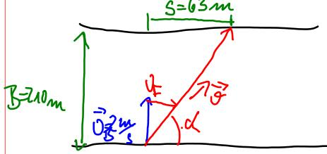
$$\left. \begin{array}{l} B = 210 \text{ m} \\ S = 63 \text{ m} \end{array} \right\} t_{\text{min}} \alpha = \frac{210 \text{ m}}{63 \text{ m}} \Rightarrow \alpha = 73^\circ$$
