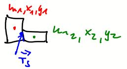
$$\vec{r}_S = \frac{\int \vec{r} \cdot g(\vec{r}) dV}{\int g(\vec{r}) dV} = \begin{pmatrix} \int x g(x, y, z) dV \\ \int y g(x, y, z) dV \\ \int z g(x, y, z) dV \end{pmatrix}$$
