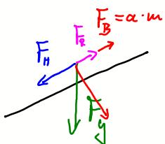
$$F_R = \mu \cdot F_N \quad j \quad F_N = F_g \cdot \cos \alpha \quad \left. \begin{array}{l} \text{Bewegung wenn } F_H > F_R \\ F_H = F_g \cdot \sin \alpha \end{array} \right\}$$
