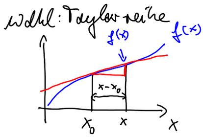
$$f(x) = f(x_0) + \frac{df(x)}{dx} \Big|_{x_0} \frac{(x-x_0)^1}{1!} + \frac{d^2 f(x)}{dx^2} \Big|_{x_0} \frac{(x-x_0)^2}{2!} + \dots$$
