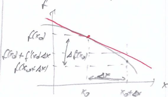
idea: Approximation of  $f(x_0 + \Delta x)$  for a given  $f(x_0)$  such that the error is of order  $O(\Delta x^2)$
