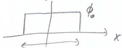
$$A(k) = \frac{\phi_0}{2\pi} \int_{-\Delta k/2}^{\Delta k/2} dx e^{-ikx} = \frac{\phi_0}{2\pi} \left[ \frac{e^{-ikx}}{-ik} \right]_{-\Delta k/2}^{\Delta k/2}$$
